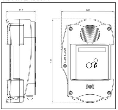
all circuits and control devices are fixed on the easy removable front plate for a very quick substitution of equipment in field
